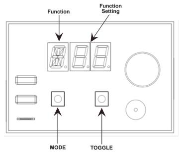
To adjust settings, press and hold MODE (yellow pushbutton on left hand side) until the Function symbol appears. Once in Adjustment Mode, keep pressing MODE until desired Function is reached (see Quick Reference Table). To change Function Setting, press and release TOGGLE (white pushbutton on right hand side) until desired Function Setting is reached (see Quick Reference Table).
