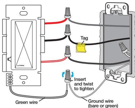
NOTE: Only one dimmer can be used in a 3-way circuit.
