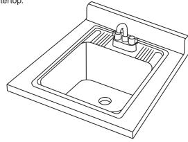
Determine the desired location of your tub on the counter top. Make sure the position will fit on the flat area of the counter top taking into account the radius curve of the back splash (if applicable). Also note clearance below the counter top to assure room for faucet and drain connections.
