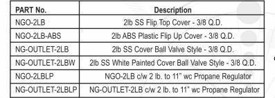
PART No.: NG-OUTLET-2LBW (Stainless Steel Painted Cover) **BALL VALVE STYLE** C.S.A. APPROVED BRASS BALL VALVE. GAS~FLO BRAND 3/8" Q.D. COUPLER.
