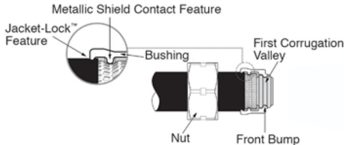
Note: Metallic shield contact feature must be utilized with FlashShield.
