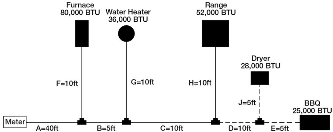
Note: Rigid pipe sized using a 0.5"WC pressure drop table, as no 2.0"WC pressure drop table for Rigid pipe is available.
