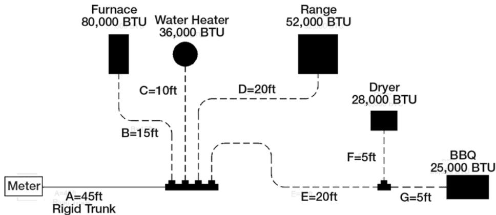
Note: Rigid pipe sized using a 0.5"WC pressure drop table, as no 2.0"WC pressure drop table for Rigid pipe is available.
