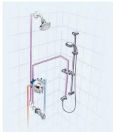
Adding a tub spout to a shower kit is simple and easy! Simply choose a diverter tub spout that matches one of the kits and pair it with a Twin Ell (03671000) to direct water from the tub spout to the shower head.
