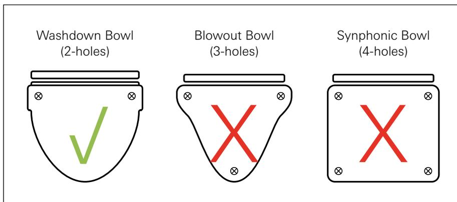
GROHE Rapid SL is compatible with any two-hole wall-hung toilet bowl offered by any major ceramic manufacturer for the utmost design freedom.
