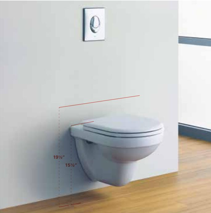
Offering superior user comfort, GROHE Rapid SL allows for installation of wall mounted toilets with a rim height ranging from 15½" to 19½". Because of the unit's flexibility, Rapid SL can meet standard and ADA compliance.
