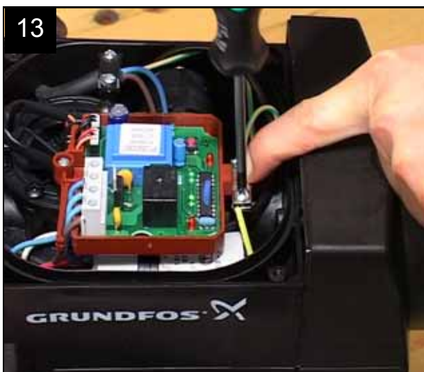
Fix the control unit and earth terminals with two screws.
