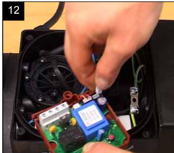
Connect the pressure switch to the control unit.
