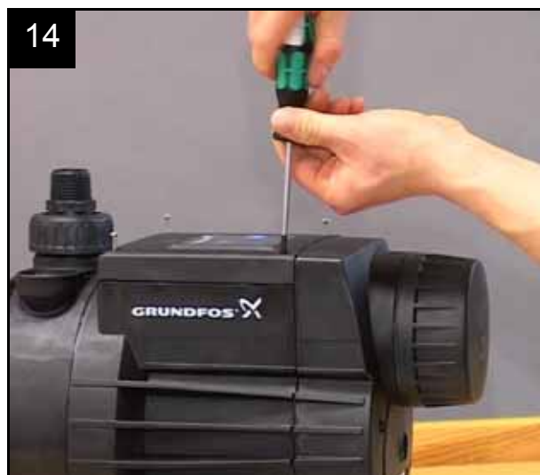
Fit the terminal box cover.
