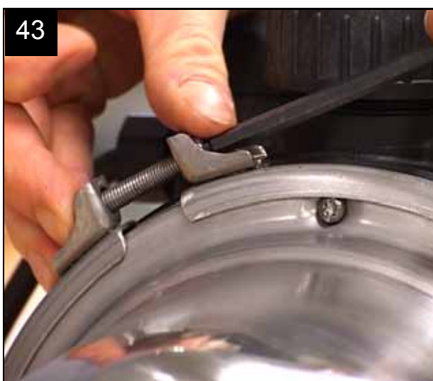
Fit the screw in the clamp and tighten.
