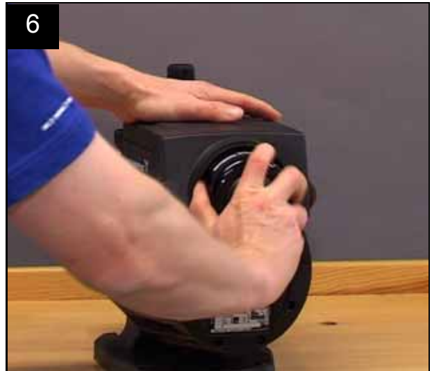
Fit the pressure tank. Tighten it by hand.
