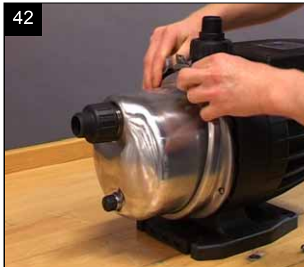
Fit the clamp on the pump.
