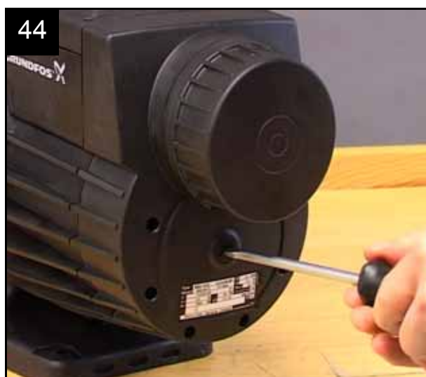
Fit the plug into the end cover.
