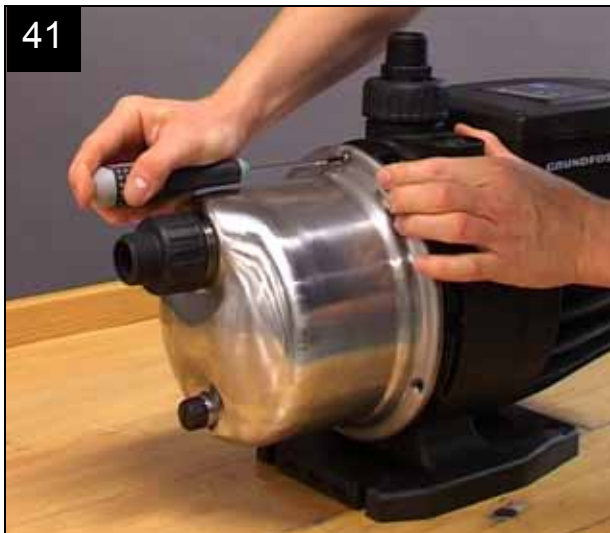
Fasten the pump sleeve.
