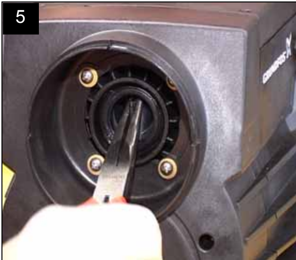
Fit the non-return valve in the pump housing.
