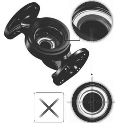
Fig. 12 Incorrectly centred sealing system
