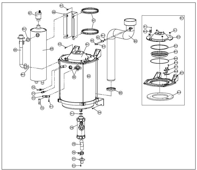
Figure 60 - Heat Exchanger Replacement Parts - 140W Models
