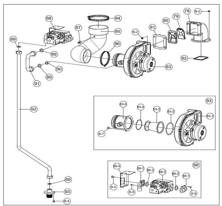
Figure 65 – Combustion System Replacement Parts – 199W Models
