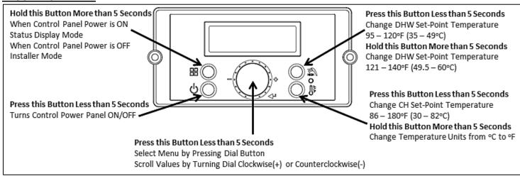
Figure 35 - Appliance Control Panel Detail
