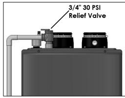
Figure 29 - Relief Valve Details
