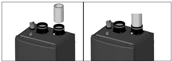
Figure 11 – Installing the 6" Length of CPVC into the Exhaust Vent Connection
