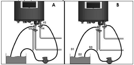
Figure 55 - A - Valve, and B - Hose Connection Details
