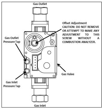
Figure 49 - Gas Valve Detail
