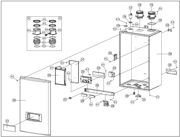
Figure 62 - Cabinet Replacement Parts - 199W Models
