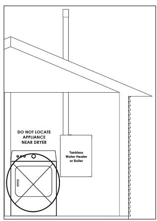
Figure 16 - Do Not Install in a Contaminated Space
