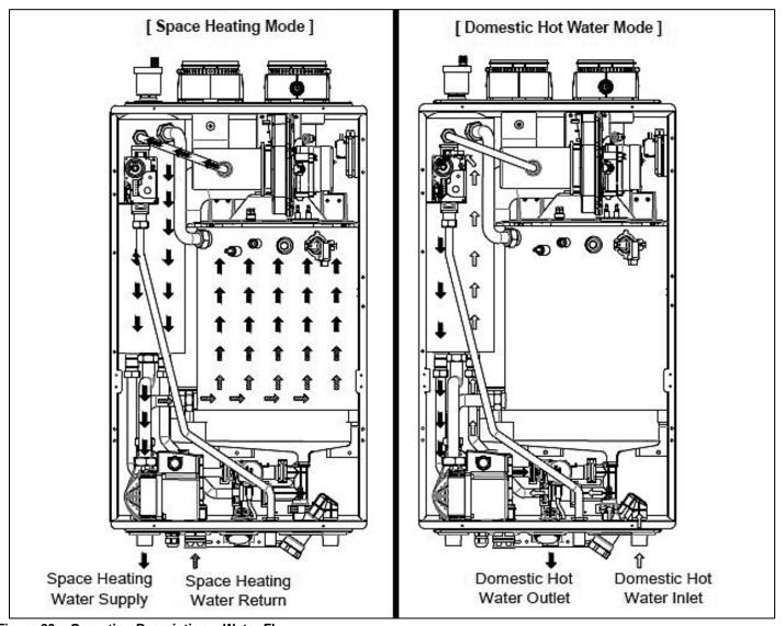
Figure 23 - Operating Description - Water Flow
