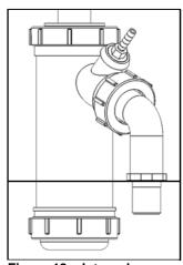
Figure 18 – Internal Condensate Trap
