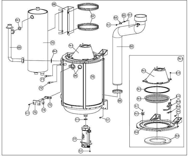
Figure 64 – Heat Exchanger Replacement Parts – 199W Models
