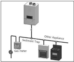
Figure 21 – Natural Gas Piping Installation – NOTE: Capacity to be Not Less than Total Capacity of Connected Appliances
