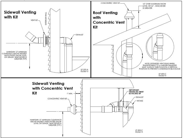
Figure 14 – Direct Vent, Vent Terminations (With Optional Kits)
