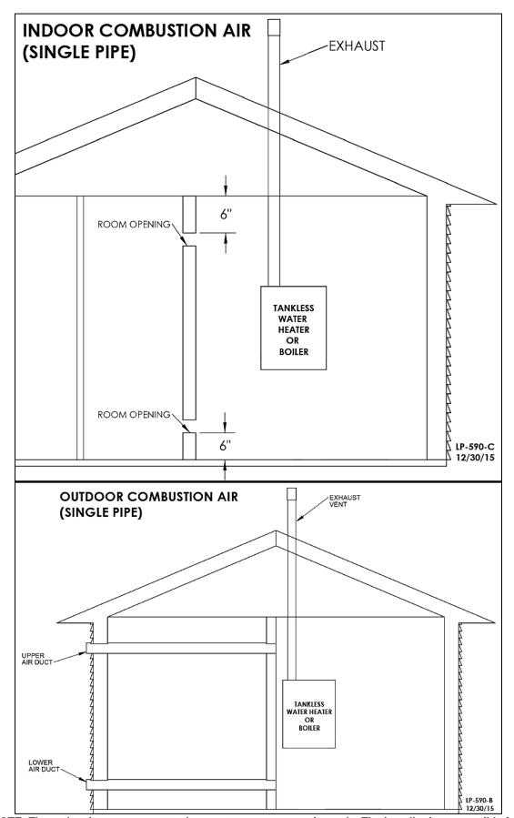
Figure 17 – NOTE: These drawings are meant to demonstrate system venting only. The installer is responsible for all equipment and detailing required by local codes.
