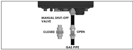
Figure 20 - Gas Line with Shut-Off Valve Detail
