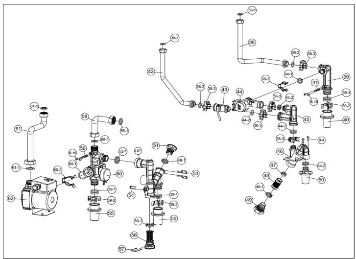
Figure 63 – Water Piping Replacement Parts – 199W Models
