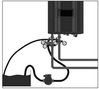
Figure 53 - Valve Detail
