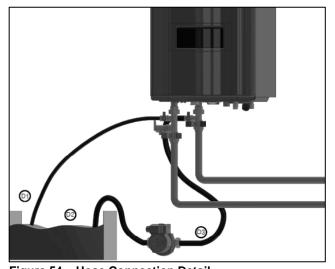
Figure 54 – Hose Connection Detail
