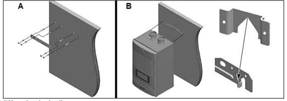
Figure 6 - Wall Mounting the Appliance
