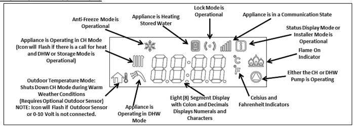
Figure 36 - LCD Display Detail
