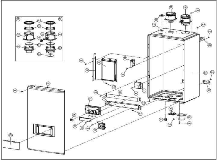
Figure 58 – Cabinet Replacement Parts – 140W Models
