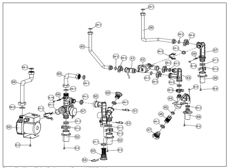
Figure 59 – Water Piping Replacement Parts – 140W Models
