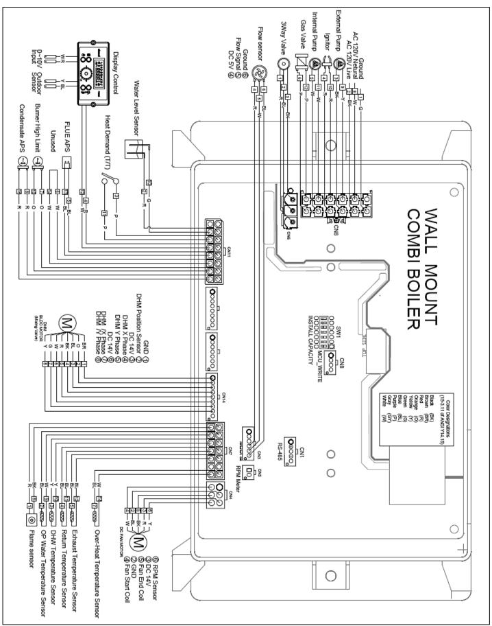
Figure 32 - Electrical Wiring Diagram
