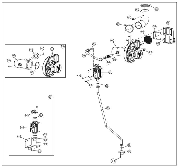
Figure 61 – Combustion System Replacement Parts – 140W Models
