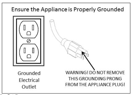
Figure 30 – Manual Power Switch and Appliance Plug Details
