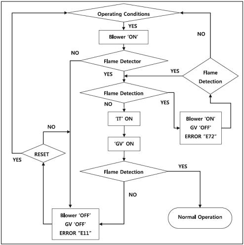
Figure 44 – Flame Detection Error Analysis Tree
