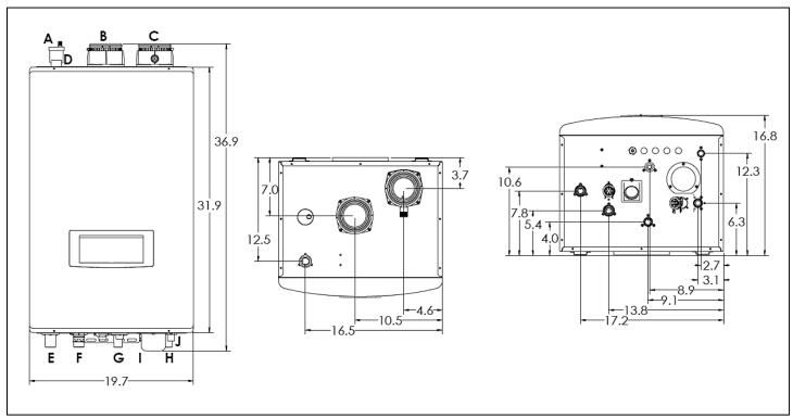
Figure 2 - 199W Specifications and Dimensions
