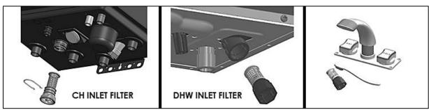
Figure 56 - Cleaning the Inlet Filter
