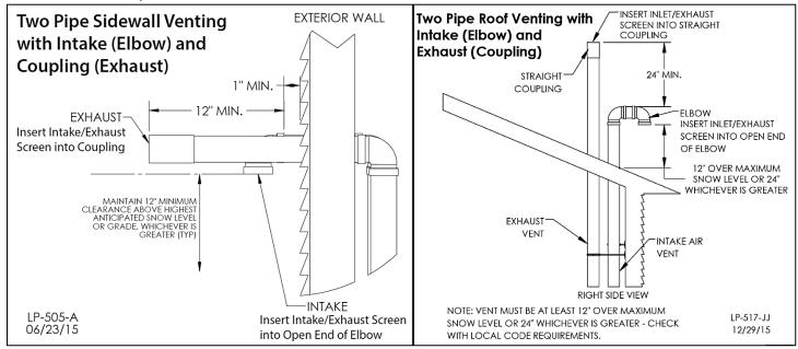
Figure 13 - Direct Vent, Roof and Sidewall Vent Terminations
