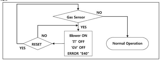
Figure 45 – Gas Detection Error Analysis Tree
