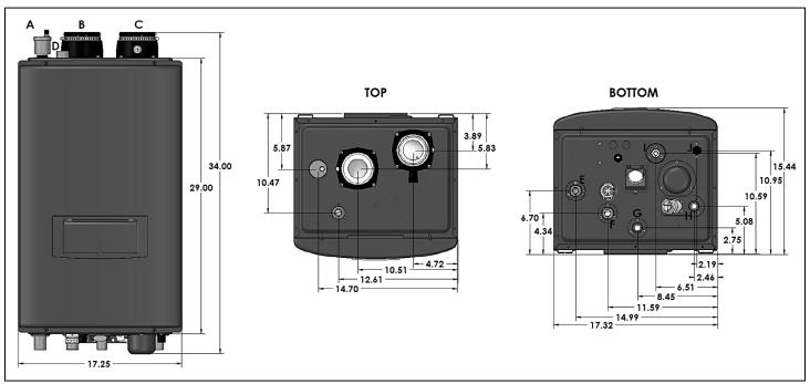
Figure 1 – 140W Specifications and Dimensions
