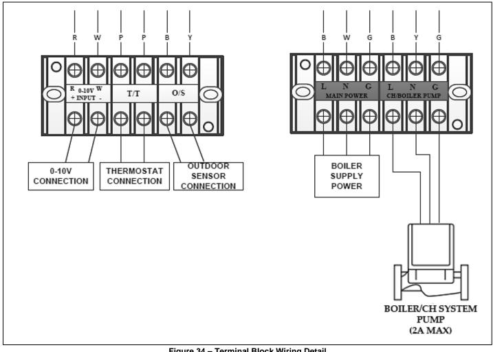
Figure 34 - Terminal Block Wiring Detail
