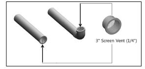
Figure 15 - Screen Installation
