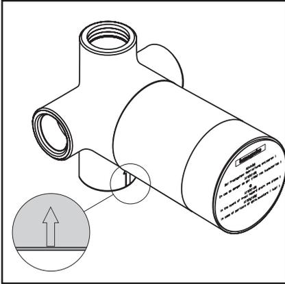
Install the valve so that the outside surface of the **finished** wall falls between the “minimum” and “maximum” lines marked on the plaster shield.
