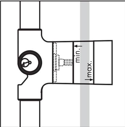
When the drywall or green board is installed, **seal the opening around the Quattro / Quattro Green with waterproof sealant.**
