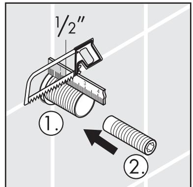
Cut the extension spindle so that it extends 1 1/4" outside the surface of the finished wall.
