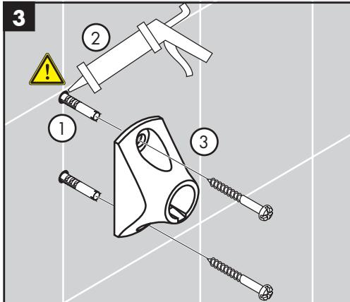
**Seal the wall around the anchors with waterproof sealant.**
