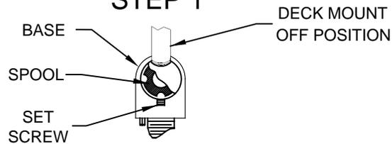
UNIT IS SHIPPED IN DECK MOUNT CONFIGURATION. TO CONVERT TO WALL MOUNT CONFIGURATION, POSITION ARM IN "DECK MOUNT OFF POSITION" AS ABOVE.
