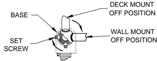
NOTE DEPTH OF SET SCREW PRIOR TO LOOSENING. LOOSEN SET SCREW AND ROTATE EYEWASH ARM 90 DEGREES CLOCKWISE (AS SHOWN) WHILE MAKING SURE TO NOT ROTATE THE SPOOL. RETIGHTEN SET SCREW IN NEW POSITION. ENSURE SET SCREW IS PROPERLY SEATED IN THE INDENT. MAKE SURE THE SET SCREW IS TIGHT AND AT ITS ORIGINAL DEPTH. ENSURE CORRECT ARM ORIENTATION BEFORE MOUNTING TO WALL. REFERENCE DRAWINGS AT RIGHT.
