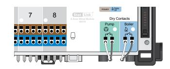
Step 11 Attach the red strain-relieving strip using the three screws to secure the pump and boiler wires to the bottom side of the module.
