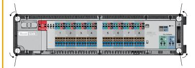
Step 2 Remove the white terminal connection board by removing the six screws shown below.
