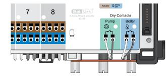
Set the actuator and boiler delay jumpers at the top right of the module by carefully removing them, and reinserting them as necessary:
