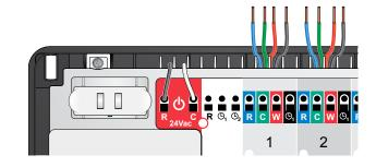
Step 8 Bend over and push all thermostat wires into the round holes at the top of the module.
