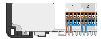
Step 10 Push in the wires for a pump and boiler (if applicable) at the bottom right of the module. Pump and boiler terminals are dry contacts.
