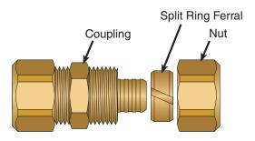
**Step 3.** Fit the nut over one of the PEX pipe end.
