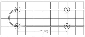
PEX tubing should be secured with tie straps every 3' (1m) on straight runs and at two points on a 180° bend.
