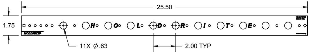
The HOLDRITE #101-18 & #101-26 is a Copper-Bonded™ steel brackets with 5/8" holes on 2" centers to support 1/2" copper tubing. The #101-18 & #101-26 position copper water supplies for sinks, water closets, and other fixtures. When soldering, heat the pipe, not the bracket.
