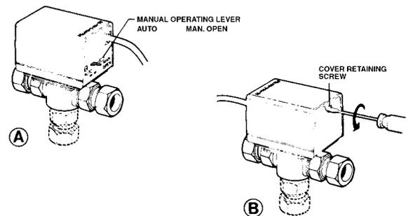
Fig. 1. Removing Cover
