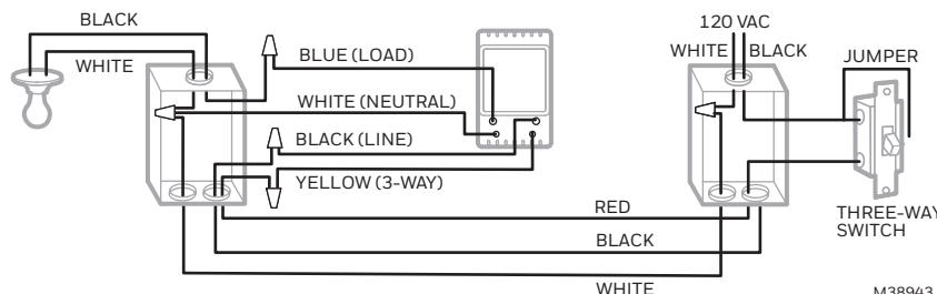
Connect the LOAD wire on the PLS750C/PLS751C to the "common" wire, which you identified when removing the old switch. Connect the NEUTRAL wire to the neutral (white) wires. Connect the LINE and 3-WAY wires to the two remaining wires. At the other 3-way switch, connect the jumper wire between the "common" screw and the screw where the LINE wire of the PLS750C/PLS751C is connected.
