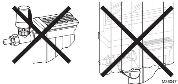
**Fig. 3. Improper installations.**
