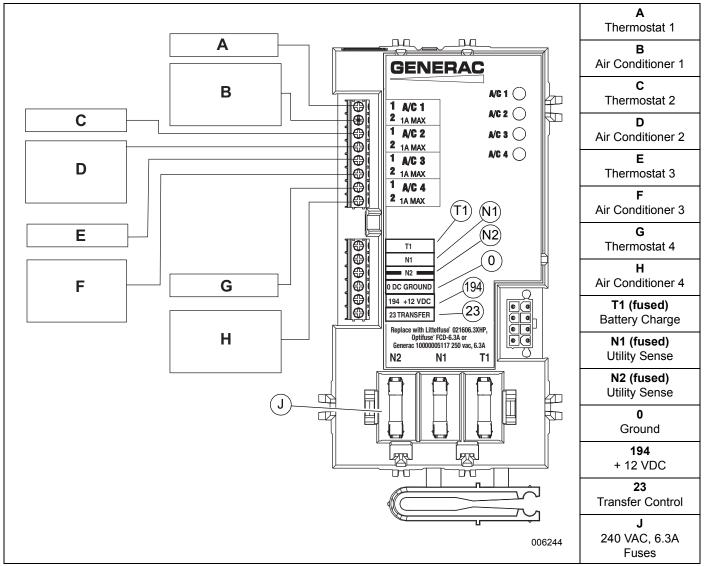
Figure 3-3. Typical SACM Connections
