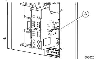
Figure 3-4. Auxiliary Contact
