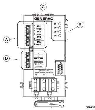
Figure 2-3. Smart A/C Module (SACM)
