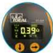
Displays Impedance of hot, neutral & ground
