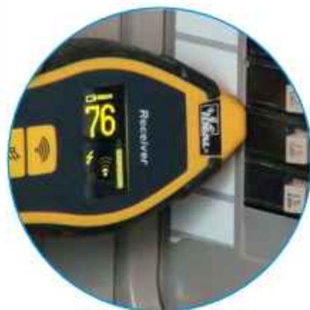
Finding Breakers or Fuses
