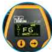
Detects and Displays false or "bootleg" ground
