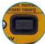
GFCI Test w/Indicator Light
