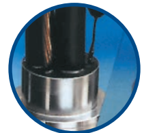
4. Pot cable (using liquid or putty)
