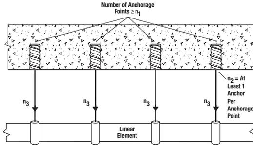
**Strength Design (Redundant Fastening):**
