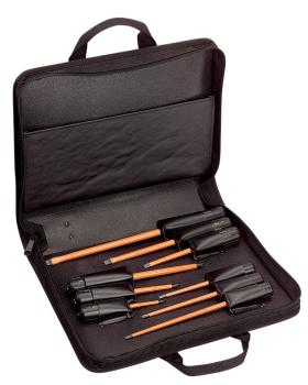
This nine piece set features assorted Klein's screwdrivers with three sizes of each tip style. Each are individually tested to exceeed the IEC 60900 and ASTM F1505 standards for insulated tools. Two layers of insulation provide protection against electric shock. The highly durable, black nylon case features a zipper enclosure, custom-fitted tool pockets as well as an extra pocket for storage of papers and other items. Made in the USA.
