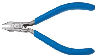
These Electronics Pliers are the smallest diagonal-cutter Klein offers for close quarter work. They feature a miniature jaw for maximum visibility in tight spaces. The sharp, pointed, tapered nose allows for precise tip cutting. The short jaws and semi-flush, beveled cutting knives permit close cutting of wire. Made of the finest U.S. steel alloy and induction hardened for long life.
