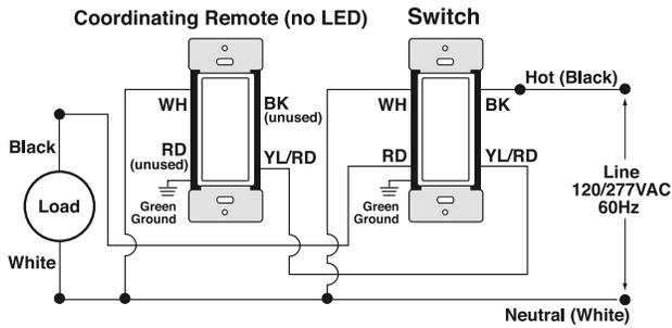
**THREE-WAY WIRING DIAGRAM**
