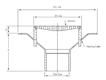
SPECIFICATION: Floway series F4000 polypropylene non-adjustable floor drain with 8-1/2" diameter strainer, sediment basket, and plain end outlet. Body with 14-1/2" diameter flange, and non-puncturing style flashing collar with weep holes.
