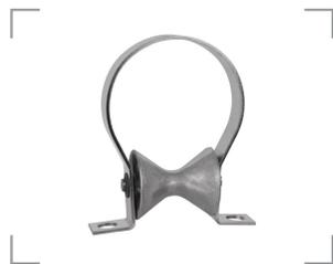
Small aluminum roller supports 1" to 3" diameter pipe. Can be mounted centrally or side by side on Blox (ROD03). Roller bracket can also be installed elevated on threaded extension rods. Use on long piping runs to allow for expansion and contraction of piping.
