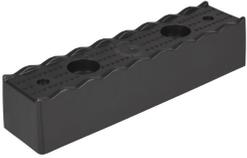
Polypropylene Height Extension fastens directly on top of Blox with two #10 screws provided. Raises Blox to 6" overall height and mimics features on top of the Blox. Extension can also be elevated for additional height using threaded extension rods (ROD03). 100lbs./45 kg max load when directly mounted to Blox or when elevated on threaded rods.
