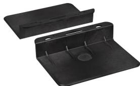
Pair of brackets secure Blox directly to roof surface. Brackets lock onto engineered mounting tabs with two #12x3/4" screws, then glue down into place with structural adhesive (ADH12/ADH12WH). Securing Brackets anchor the Blox into final installed position and protect against movement due to moderate wind, water, and snow loads.
