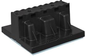
Polypropylene copolymer roof top support block engineered to support load directly attached with straps, clips or clamps, or the Blox easily adapts with accessories listed below. Includes on-board galvanized strap for short piping runs. Install every 7' along piping. 250lbs./113 kg max. static load single point loading. 350lbs./158 kg max. static load with strut applied. Bundled in convenient 8 pack totes.
