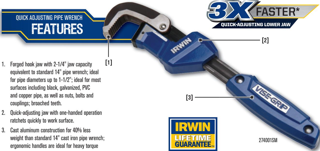
1. Forged hook jaw with 2-1/4" jaw capacity equivalent to standard 14" pipe wrench; ideal for pipe diameters up to 1-1/2"; ideal for most surfaces including black, galvanized, PVC and copper pipe, as well as nuts, bolts and couplings; broached teeth.
