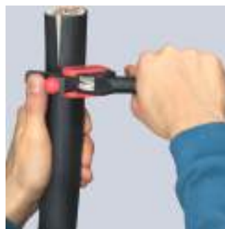
Turning the tool for circumferential cut
