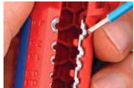
Stripping single conductor wire
