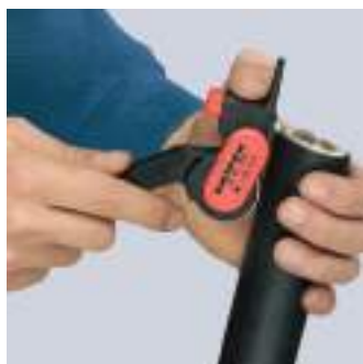
Setting the tool for longitudinal cut
