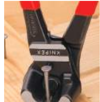
Almost flush cutting of bolts, nails, etc.
