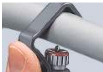
Setting the tool for circular cutting
