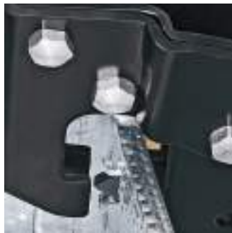
The punching tool is pressed through the metal section sheets
