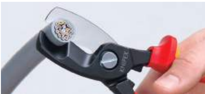
Initial cut: using the front cutting edge to cut the insulating sheath on larger cable diameters leaves an ergonomic handle opening width.
