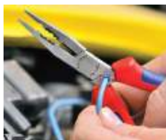
Crimping 20-14 AWG (0.5 to 2.5 mm 2 )
