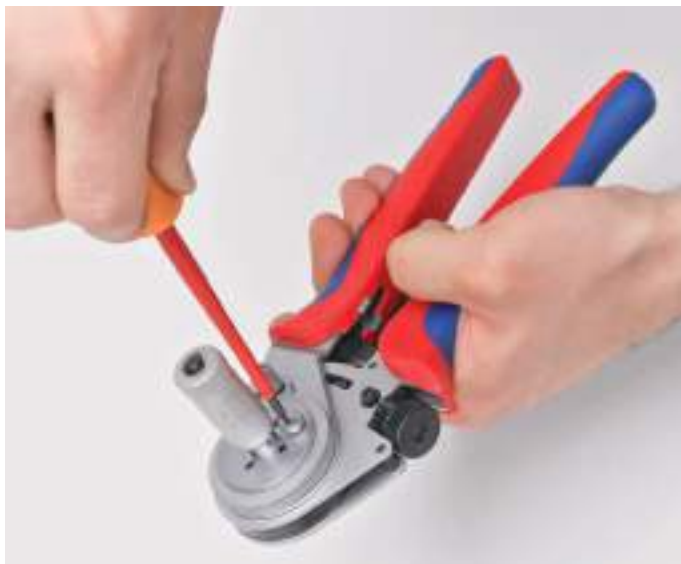
Locator 97 59 65 2 for four-mandrel crimping pliers, adjustable in length and diameter for various plugs
