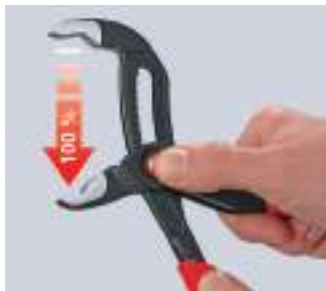
Press the button – open pliers completely
