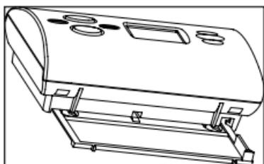
1. Remove the bracket/back cover from the unit by sliding a screwdriver between the unit and the cover at the recess in the center of the unit. This allows access to the back of the unit.
