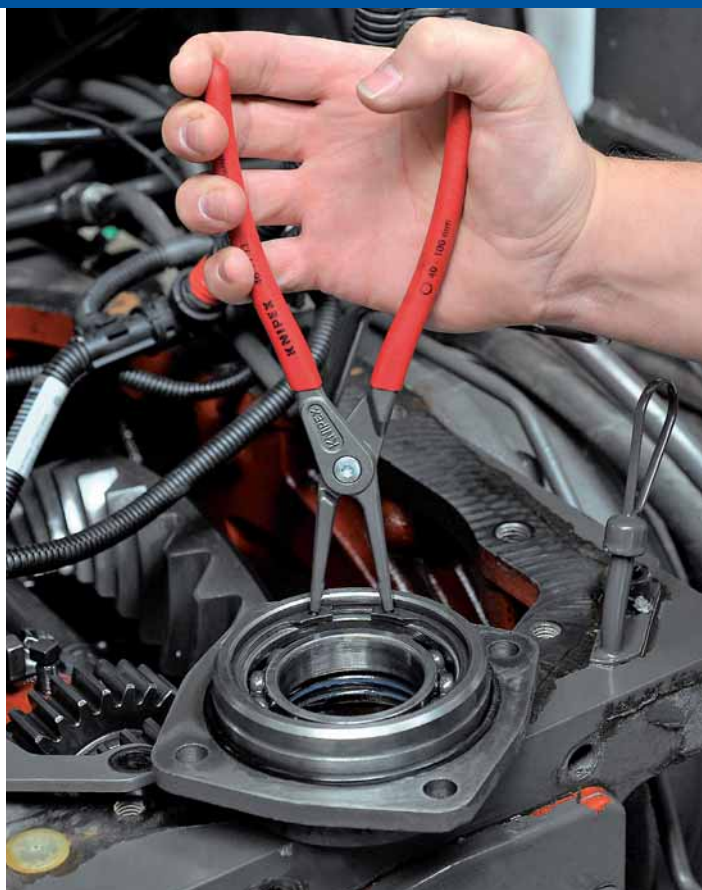
Precision Circlip Pliers to assemble internal circlips into bores
