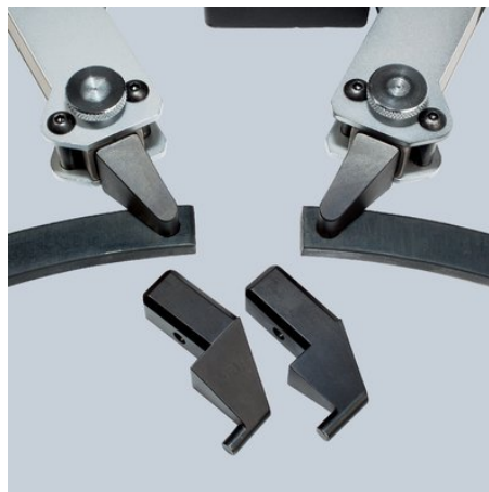
replaceable inserts for internal and external circlips
