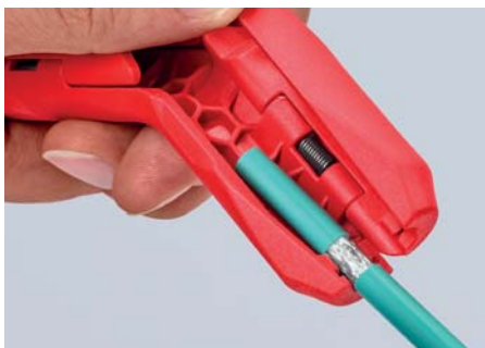
Stripping of a data cable
