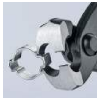
Using the side press jaw
