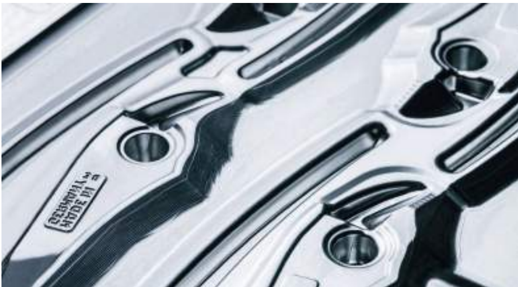
Forging die for the high leverage diagonal cutters with forged-in axle.
