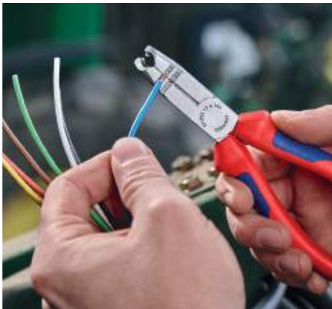
Wire stripping holes for 1.5 and 2.5 mm 2 conductors
