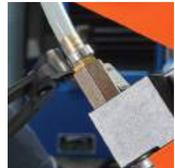
Sealing the hose connection on central lubrication
