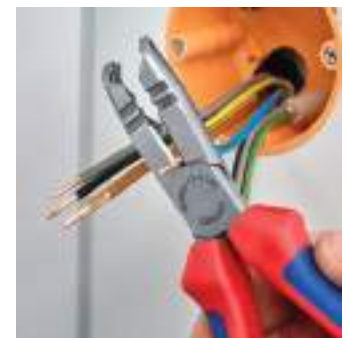
Cutting when shortening single conductors
