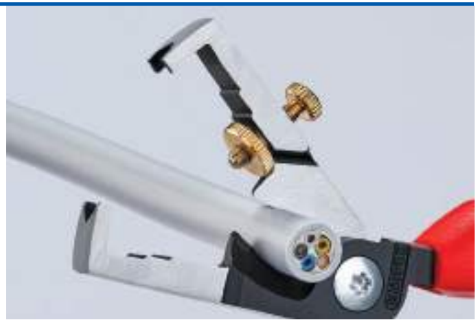
Induction hardened shear blade with precisely ground cutting edges for crushing-free cutting of copper cables up to 9/16" (15 mm Ø) (5 x 2.5 mm²)
