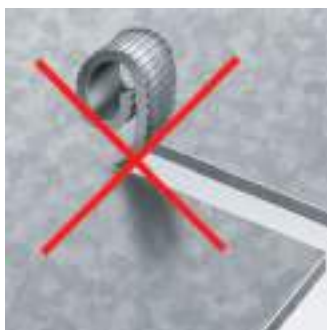
Notching without chip breaking
