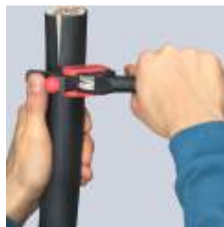
Turning the tool for circumferential cut
