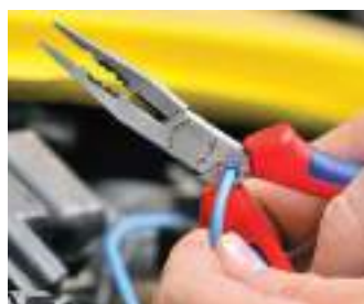
Crimping 20-14 AWG (0.5 to 2.5 mm 2 )
