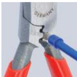
Crimping 20-14 AWG (0.5 to 2.5 mm 2 )
