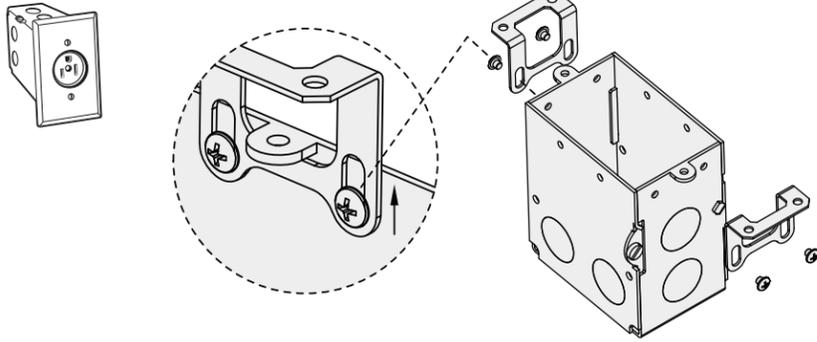
**DUPLEX RECEPTACLE** - Mount brackets on **SIDES** of floor box in the "DOWN" position.
