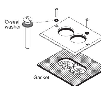
Torque mounting plate screws to 9 in-lb.
