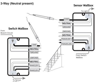
NOTE: Sensor must be installed in the location where the load wire is.
