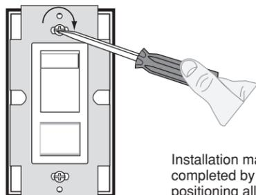
Installation may now be completed by carefully positioning all wires to provide room in wall box for dimmer. Mount dimmer into box with mounting screws supplied. Attach wallplate.
