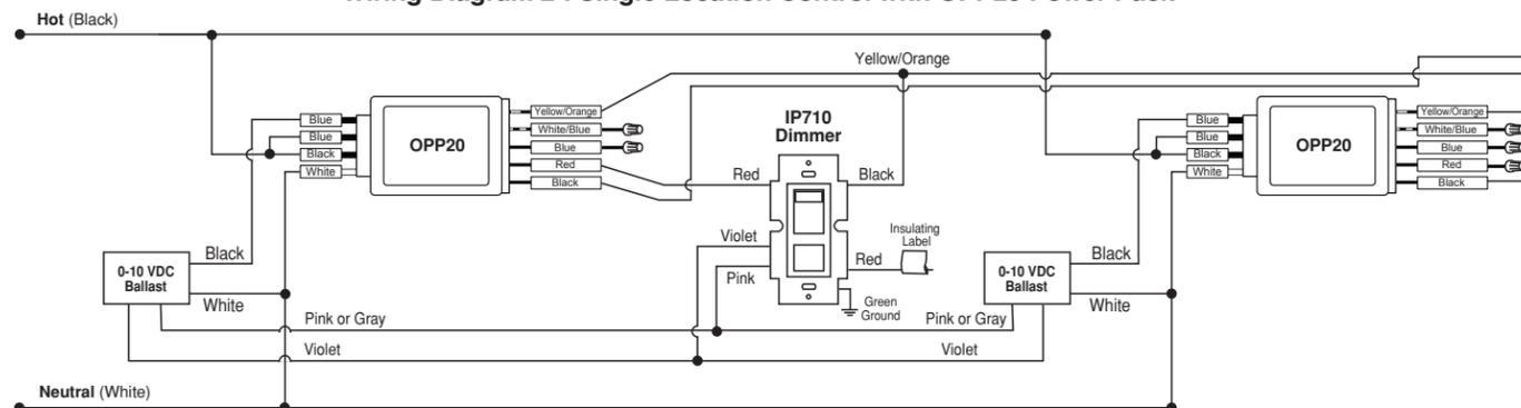
**Wiring Diagram 3: Two Location Control**
