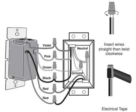
Connect wires per **WIRING DIAGRAM 3** (shown on page 2) as follows:
