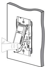
b. With the front faceplate of the sensor removed, push both buttons on front of sensor simultaneously for 10-15 seconds (note: after 5 seconds, a light will blink BLUE and then alternate between BLUE and RED) and release when the Locator Light is blinking GREEN.
