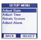
**Adjust Date Screen -** The Adjust Date screen allows you to set the date of the SPD. Use the UP and DOWN buttons to adjust the value in the selected field until you have the correct value. Press the left button (NEXT) to advance the cursor to the next date field. Press the right button (DONE) to finalize and save your changes to the SPD memory. The Setup Menu screen automatically appears.
