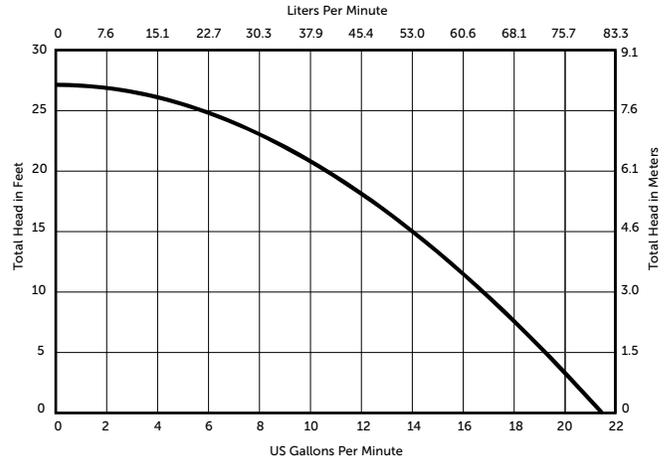
For proper performance, tank inflow cannot exceed pump discharge capacity at the installed head level.
