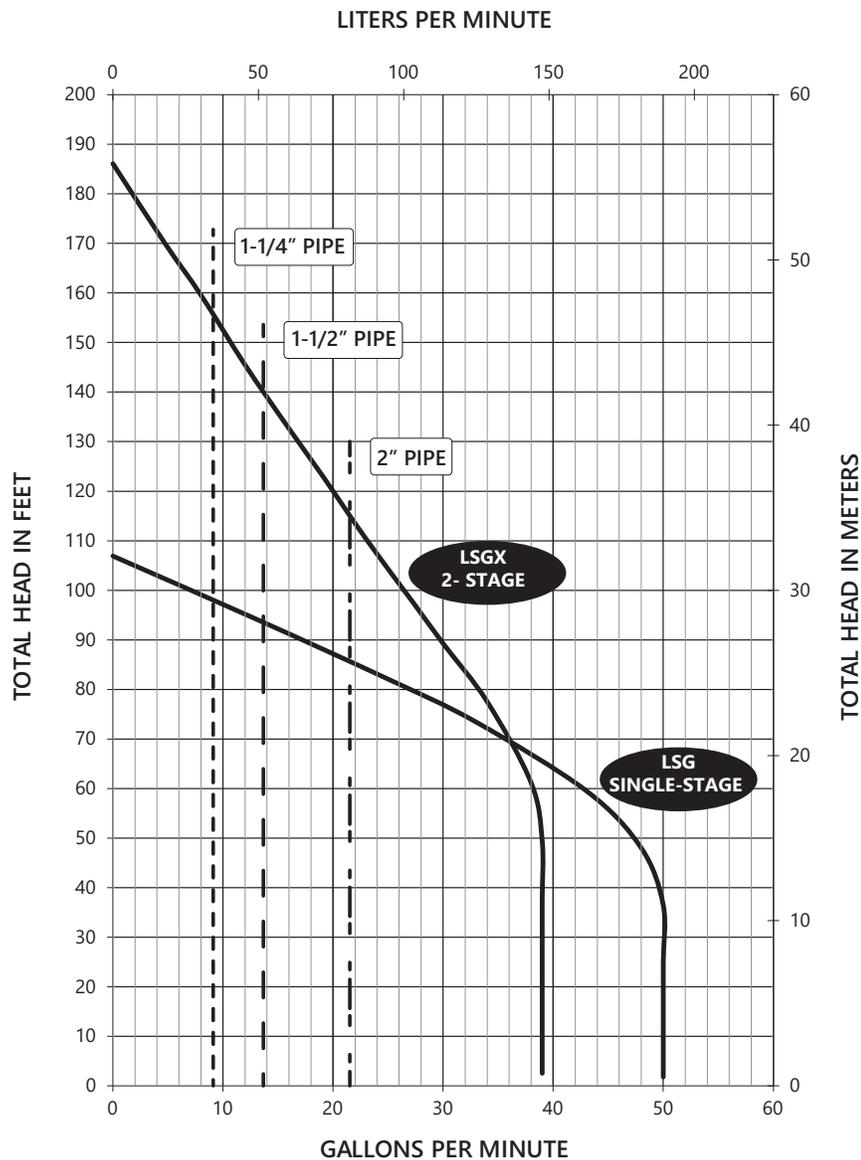
**Note:** The 2-stage LSGX202-RE and LSGX202-REX will meet the pressure specifications of E/One Series GP200, GP2000 and Extreme Series pumps. However, these progressive cavity designs have the capability to develop higher pressure than the single-stage grinders LSG202-RE and LSG202-REX.
