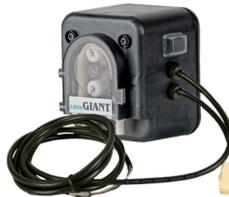
TPT Series Pump is controlled by changes in temperature of the air moving through the air condition coil. Thermal sensors constantly measure difference of "air in" and "air out". When temperature difference reaches 10 °F, pump starts. Sensor cable is 6.5 ft.
