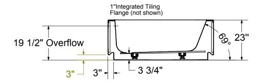
This technical drawing is universal for all ModulR bathtub configurations. (Left/Right Corner & Wall-mounted)
