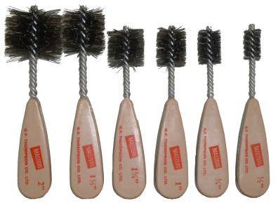
MASTER® HEAVY DUTY FITTING BRUSHES are the highest quality brushes available for cleaning copper fittings. This heavy duty unit is made of heavy gauge galvanized stem wire and oil tempered, high carbon level fill wire with double stem (4 wire) double spiral construction. The 4 wire stem is firmly secured in the hand-contoured handle.
