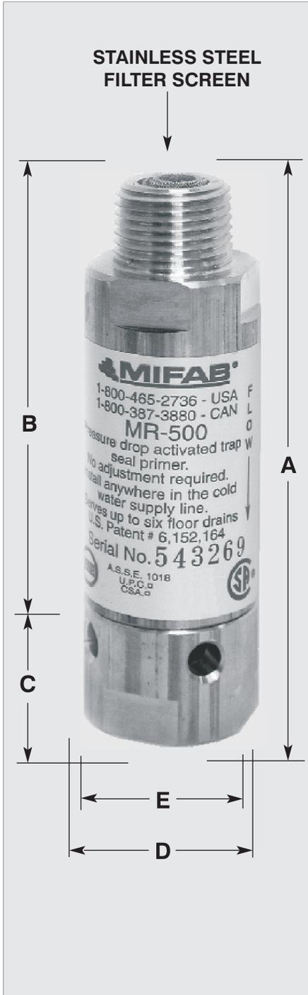
**SPECIFICATION:** MIFAB model MR-500 pressure drop activated brass trap seal primer, with inlet opening of 1/2" (13) male N.P.T. and outlet opening of female 1/2" (13) N.P.T. Complete with four view holes and removable filter screen. Serves up to 6 floor drain traps and requires no adjustments and no air pre-charge.
