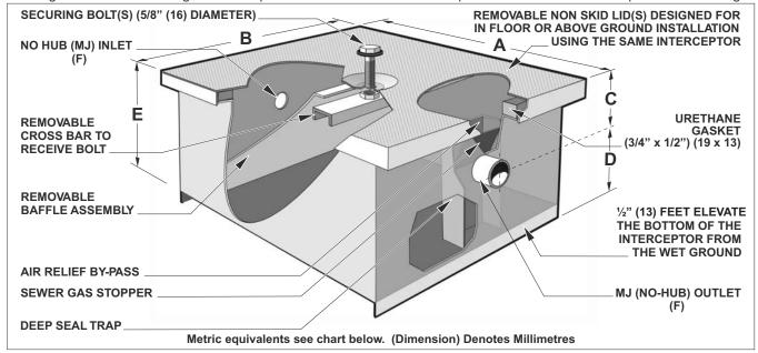
**Note:** The "C" dimension detailed above is from either the middle of the inlet or the outlet to the top of the interceptor. The inlet and outlet dimensions are always the same.
